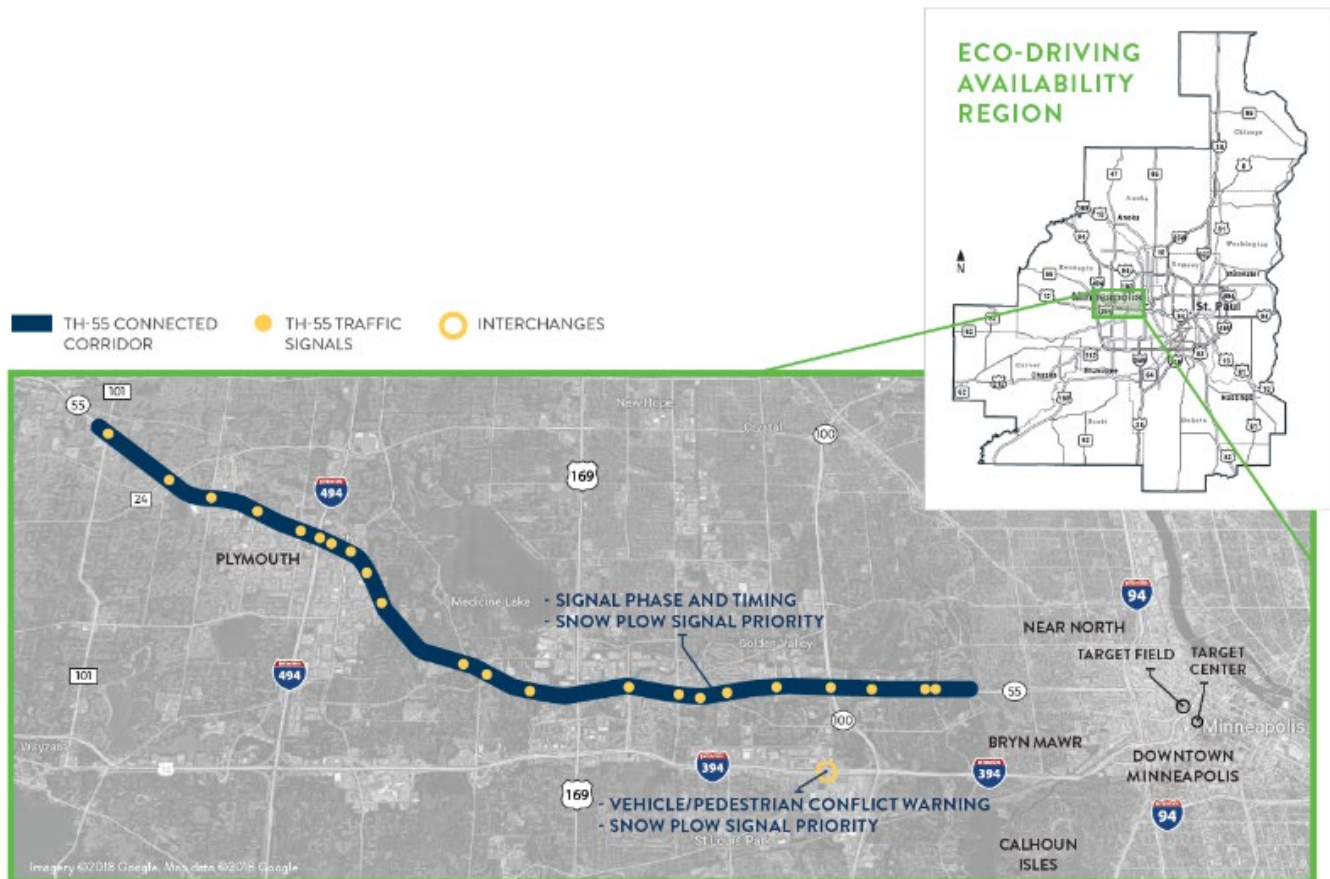
Figure 1: Trunk Highway 55 Connected Corridor between Minneapolis and I-494
